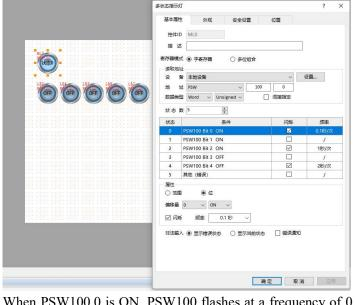
When PSW100.0 is ON, PSW100 flashes at a frequency of 0.1 seconds per time and the font display status is 0.
